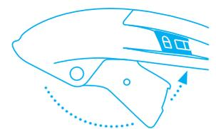
Finally, push the lever back into the handle until you **hear it click into place**.
